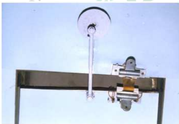
Figure 2. Apparatus for determination of folding endurance of the Patch.
